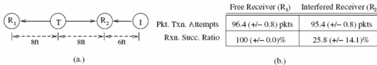
Fig. 1. (a.) A simple topology to show the hidden terminal problem; (b.) the 75% packet loss from T to R 2 is a huge energy penalty to the network.
