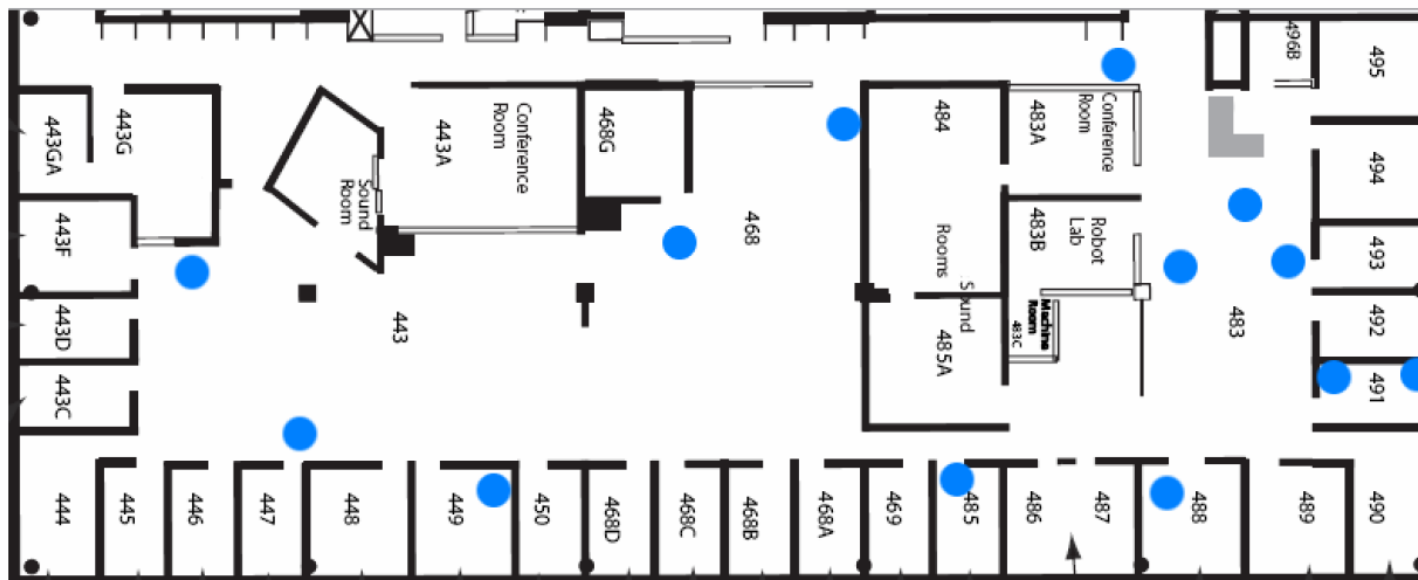
Figure 4: Testbed Topology. The figure shows the testing environment. The dots mark the locations of the GNURadio nodes.
